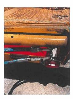
• Add safety chains to existing mounts with safety clasp hooks.
